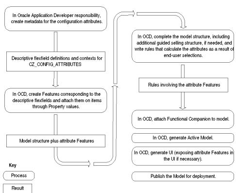
Figure 1–1 Control and Data Flow at Design Time for Output
